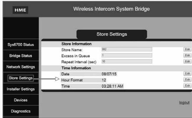
13. **Excess in Queue** alert tones are sounded in the ceiling speaker if too many customers are in queue and more order takers are needed. Click **EDIT** to access the *Excess in Queue* settings. Use the pull-down to select a number. The range is 1 to 20, but the setting should be set at “1”. Click **SAVE**.
