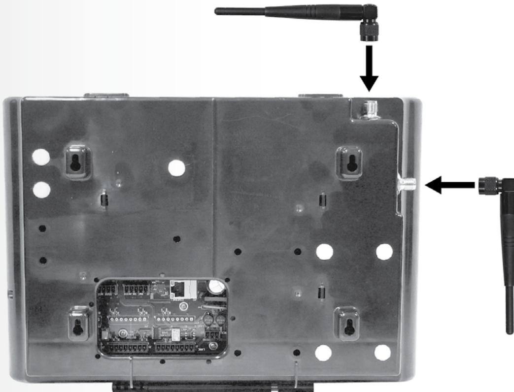
Figure 4. Antenna mounting
