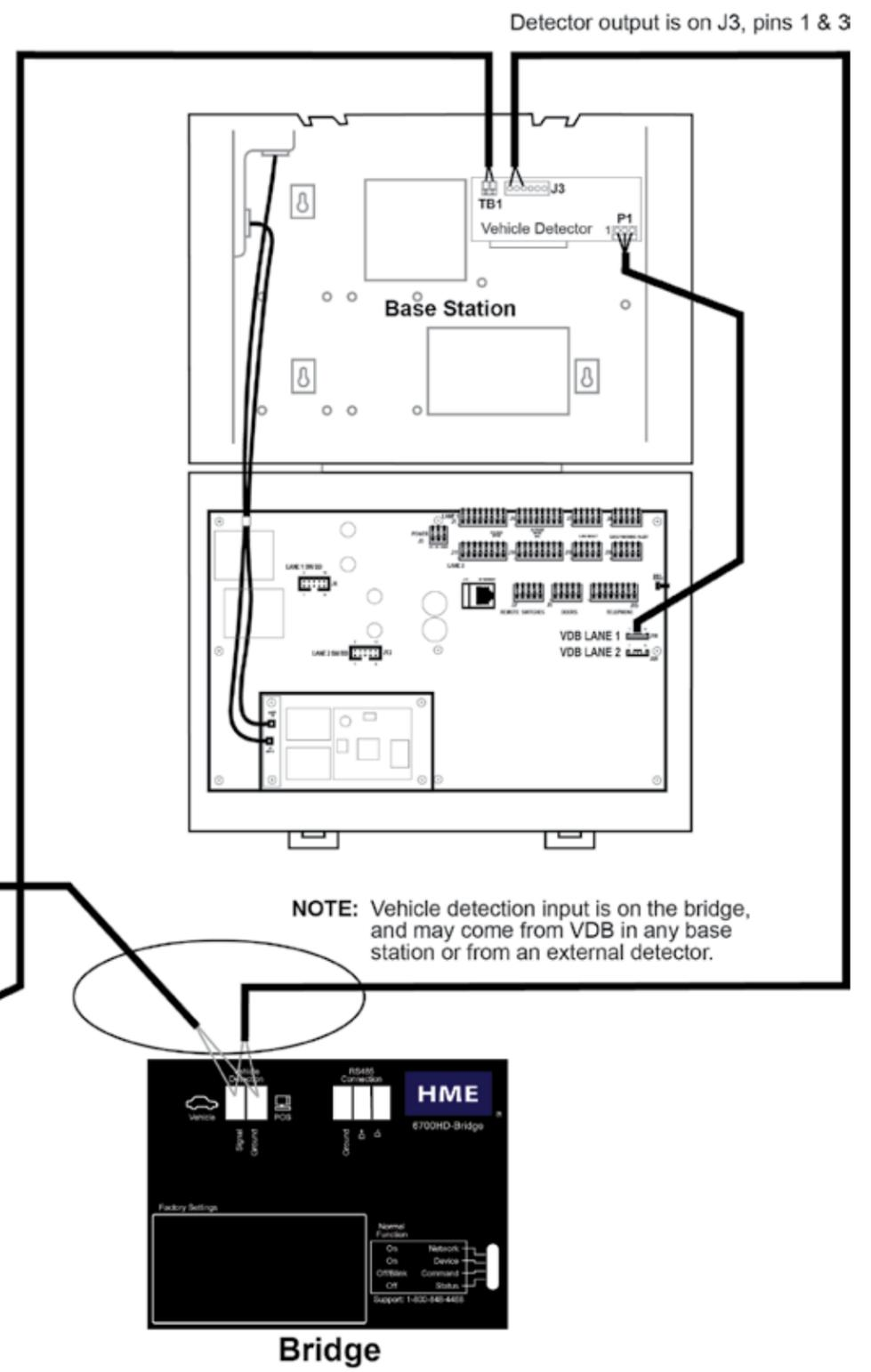
**System 6700HD Wiring Diagram for Speaker/Microphone and Vehicle Detector in Drive-Thru Lane**
