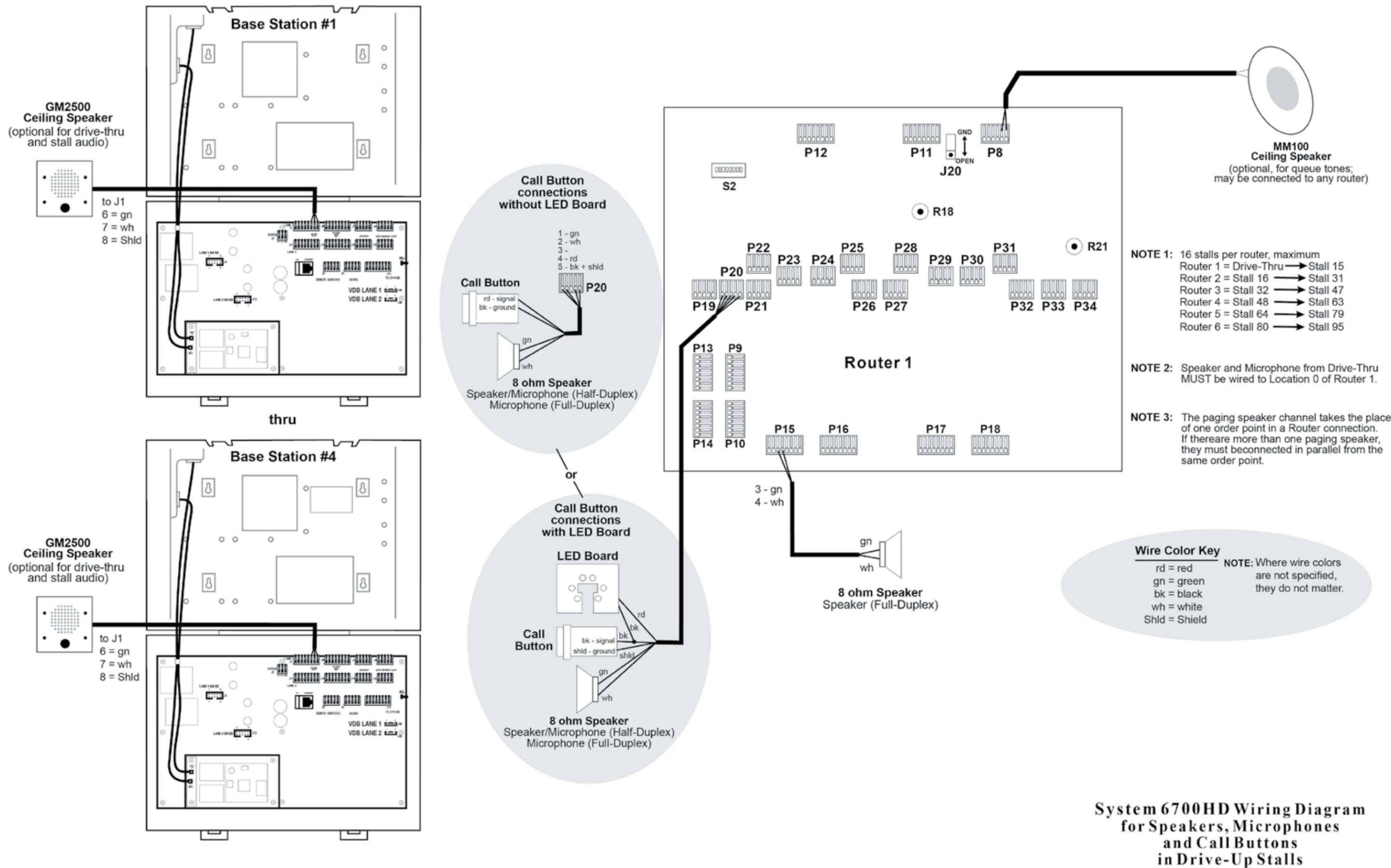
Figure 22. Speakers, Microphone and Call Buttons in Drive-Up Stalls
