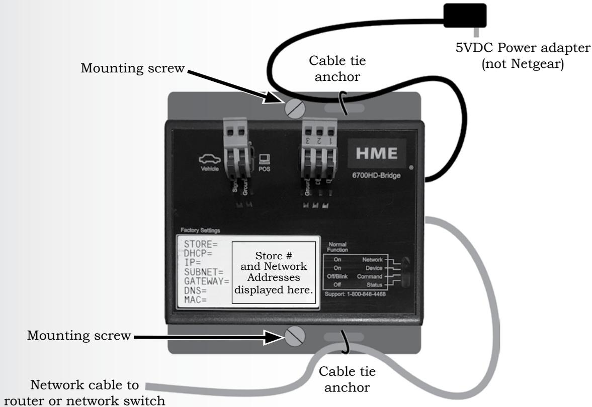
Figure 16. 6700HD Bridge mounting and cable connections
