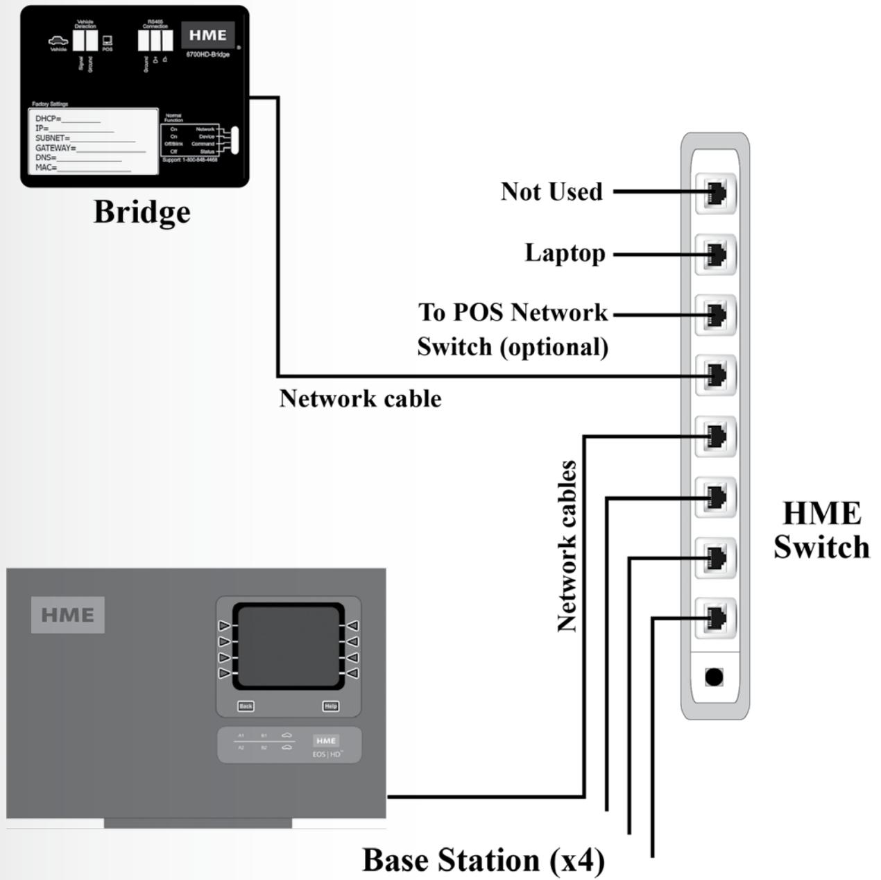
Figure 17. HME 6700HD Bridge wiring diagram
