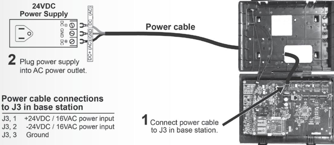
Figure 7. Power supply connection to base station
