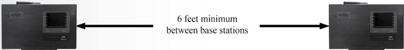
Figure 5. Distance between base stations
