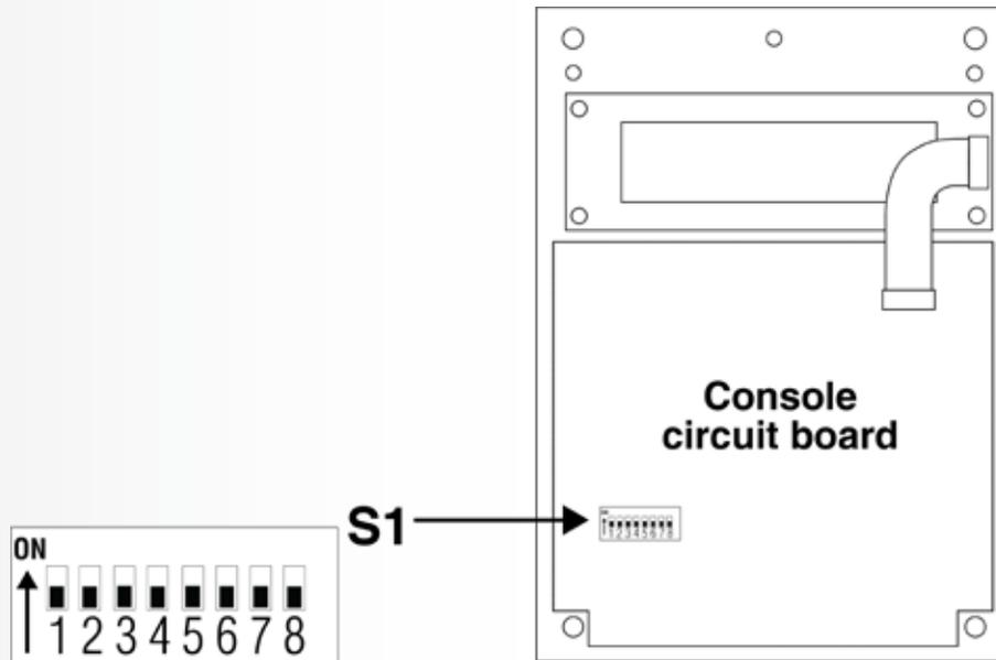
Figure 14. Console DIP switch
