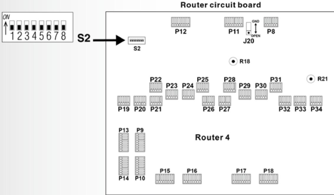
Figure 9. Router DIP switch
