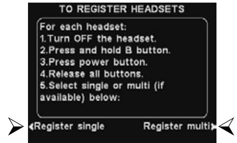
5. Activate Registration mode by pressing and holding the **B button** and then pressing the **Power button** (red) simultaneously. Once the power light starts to flash, release the buttons.
