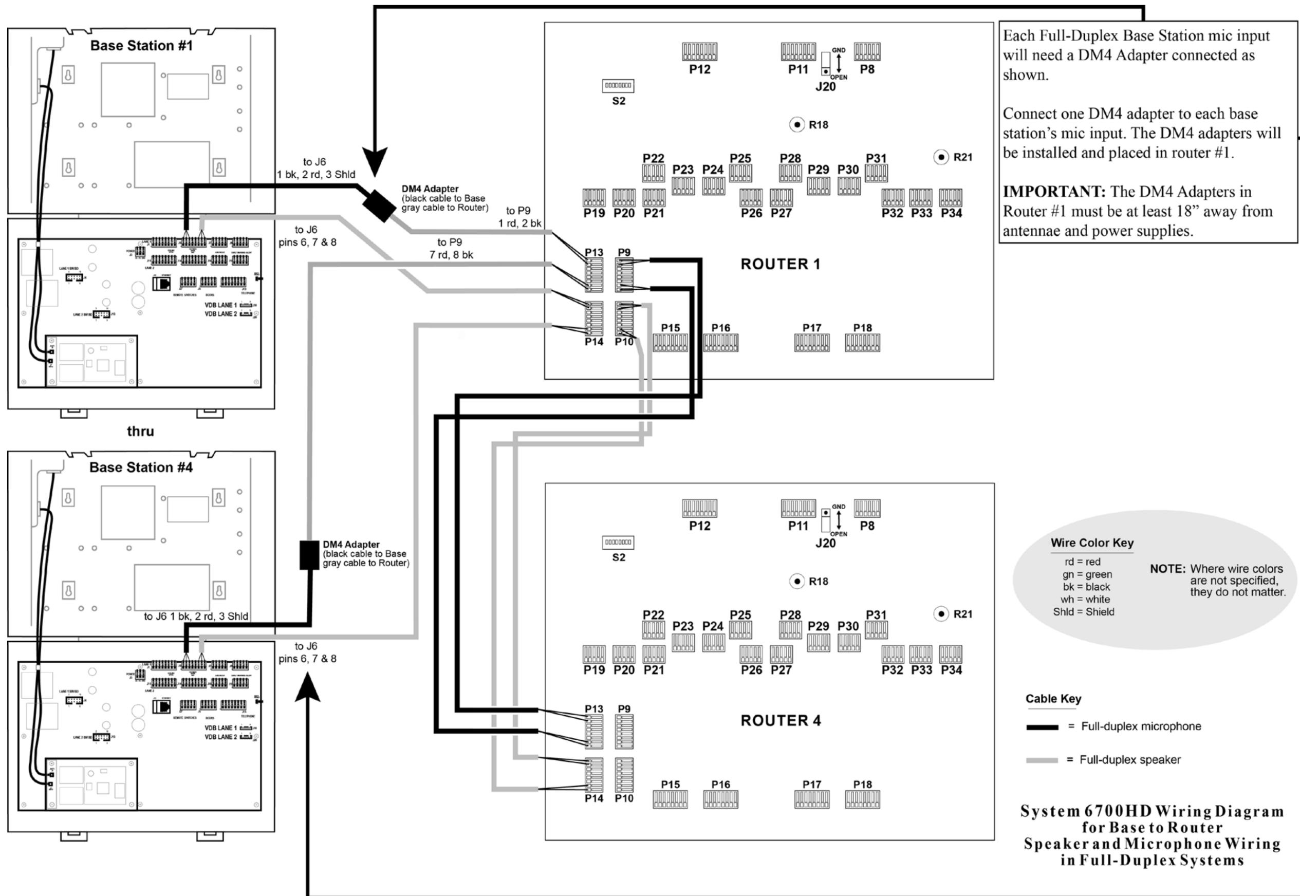
Figure 21. Base to Router Speaker and Microphone Wiring in Full-Duplex Systems
